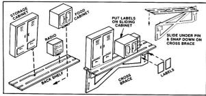
Apply labels to storage cabinets\*, and then snap cabinets to shelf and install into position on rear cross back brace. (See Illus.)
