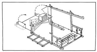
6. Fold up back and fold the flaps over corner post.
