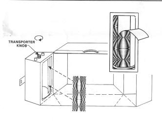
(2) Now take the large Yellow & Black pattern labels (each label is cut into 3 strips) and remove one strip from the release paper and attach it to one side of the Transporter Compartment. (See Illus.)
