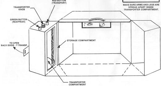
(6) To operate Transporter, place figure in the transporter compartment. Make sure that the arms and legs are spread apart inside transporter compartment. Spin the Transporter knob on the top to activate the Transporter. Press the Green button and the figure will dissappear. (The figure can be removed through the back door). To bring the figure back spin the Transporter knob and press the Red button, the figure will reappear. (See Illustration)
